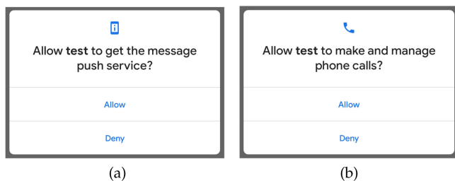
Fig. 1. Grant or deny a runtime custom permission to the app test in Android 10. (a) The custom permission is not in any group. (b) The custom permission is in the PHONE group.
